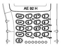
Your scanner's keys have various functions labeled on the key tops and below the keys.
