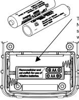
The switch is factory preset to NiMH battery and covered by a sticker. Remove the sticker if You want to use alkaline batteries
